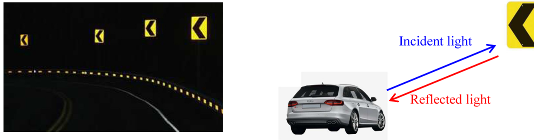
Fig. 6. Traffic signs made of retro-reflective surface appear bright at night.
